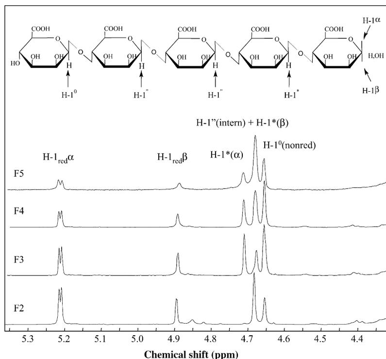
Fig. 2. H-1 region of a 400 MHz  $^1H$  NMR spectra of oligomannuronic acid standards F2–F5 obtained from a 3 h partial hydrolysis. The prefixes 'red, non-red and intern', respectively denote the reducing end, non-reducing end and internal residues. The numbers correspond to the proton assigned to the signal.
