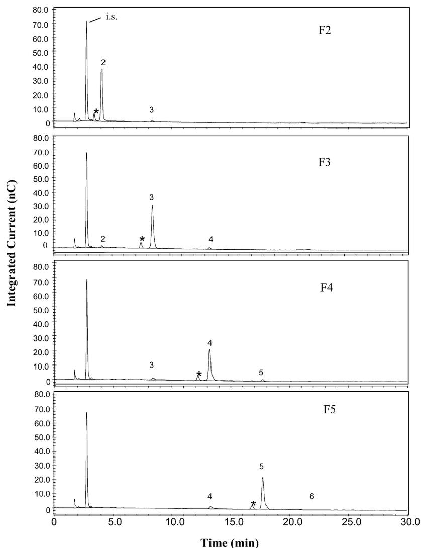
Fig. 7. HPAEC-PAD of oligomannuronic acid standards F2–F5 separated on an IonPac AS4A column using an acetate gradient in NaOH. The symbol (\*) represents an unidentified peak. Initials i.s. denote the internal standard. Peak labels (2–6) refer to the respective assigned degree of polymerisation of oligomers responsible for the peak.
