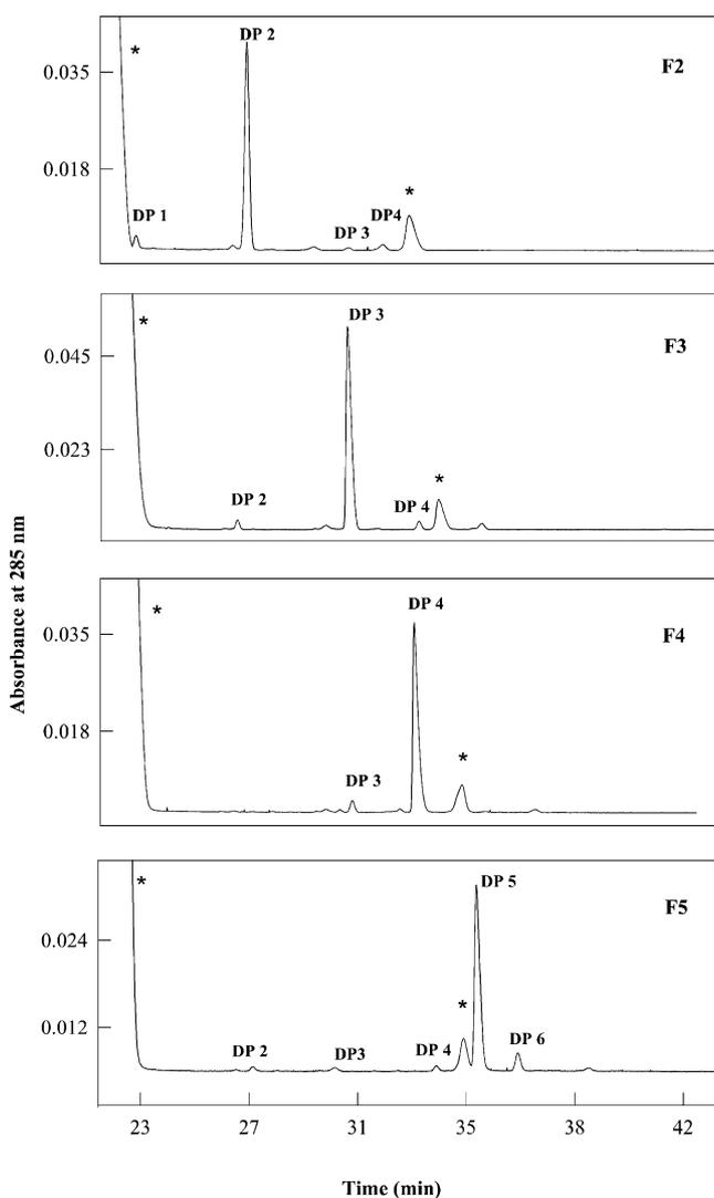
Fig. 4. MEKC-UV electropherograms of ABN-derivatised oligomannuronic acid standards F2–F5 obtained from a 3 h partial hydrolysis and detected by their UV absorbance at 285 nm (75 mM SDS in buffer). The symbol\* denotes absorbance from free ABN. The acronym DP and the respective integer (1–6) refer to the assigned degree of oligomer polymerisation for each peak.
