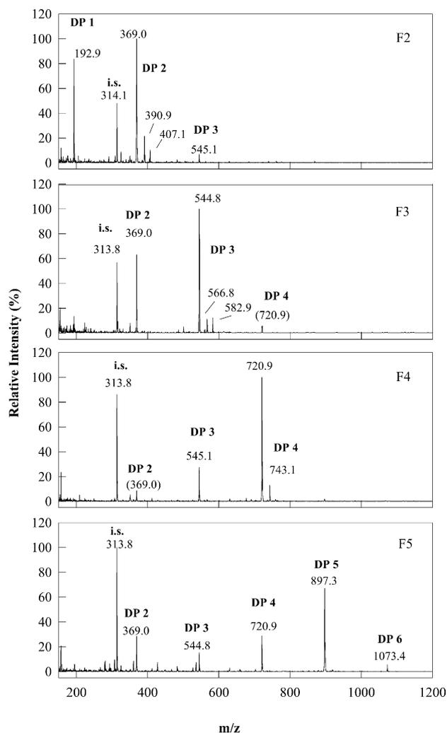
Fig. 3. Negative-ion ESI mass spectra of oligomannuronic acid standards F2–F5 obtained from a 3 h partial hydrolysis. Initials i.s. denote the internal standard, while DP and the respective integer (1–6) refers to the degree of oligomer polymerisation.
