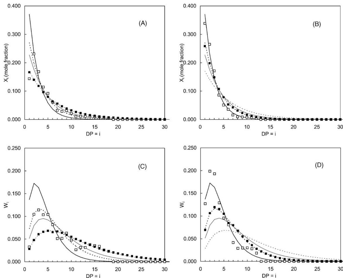
Fig. 6. Number (A and B) and weight (C and D) distribution of oligomers in mannuronic acid hydrolysis mixtures that were hydrolysed for 5 (A and C) and 8.5 h (B and D) and analysed directly. Filled squares (■) are data from HPAEC-PAD while open squares (□) are from MEKC-UV. Theoretical Kuhn distributions for  $DP_n = 2.7, 3.7, 4.4,$  and  $5.9$  are plotted as black solid, black dashed, grey solid and grey dashed lines respectively.
