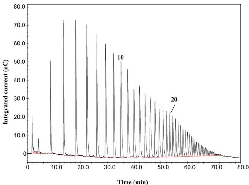
Fig. 8. HPAEC-PAD of an oligomannuronic acid 3 h hydrolysis mixtures without an internal standard and separated on an IonPac AS4A column using an acetate gradient in NaOH. Peak labels refer to the respective assigned degree of polymerisation of oligomers responsible for the peak.
